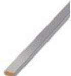
Neutral busbar, width: 10 mm, height: 3 mm, DIN VDE 0611-4: 1991-02, material: Copper, tin-plated, length: 1000 mm, color: silver
